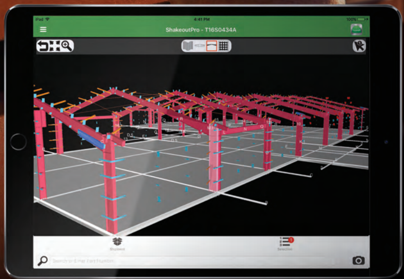
SCAN PART | The scanned part is instantly highlighted in your project model. You can scale, rotate and turn off and on layers to best view the part and determine where to stage it.
